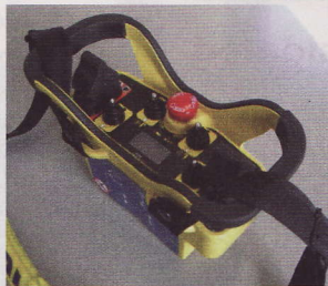
The radio remote control supplied as standard on Bluelift’s 22m machines also operates the engine selection, start/stop, lifting movements and the emergency lower procedure.
