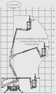
With outrigger pads removed. Pads increase width by 100 mm and height by 30 mm in stowed position.
